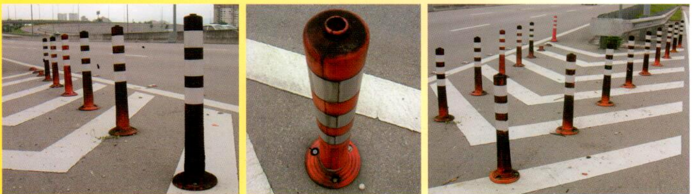
When exposed to harsh weather conditions, other reboundable delineators turn black due to fungus attack.
